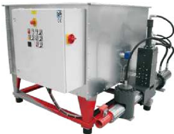
Briquetting press AP 575 with strand length monitoring
