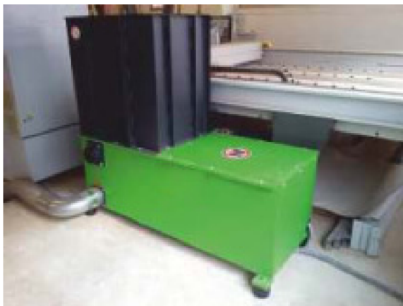
EZ 6/1 next to a panel for the crushing of particle board and plywood panels remains
