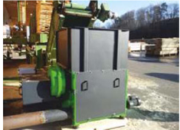
EZ 10/2 with 37 KW, filled with scrap wood on the conveyor belt, material discharge with discharge to the slate floor conveyor
